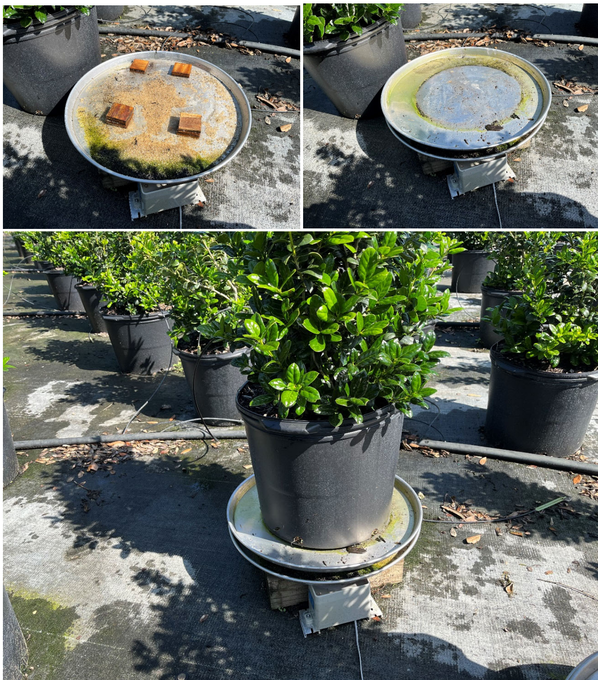
Fig. 3. Double pans were used to collect leachate and direct it to a tipping bucket rain gauge under hole in bottom pan. The bottom pan (top left) angled downward to the tipper has a handful of sand located above and around the drain hole to slow the leachate and filter out debris. The top pan (top right) is angled in the opposite direction using small wood pieces (placed on bottom pan) so that the leachate from top pan drains near the elevated edge of the bottom pan. Lower photo of Dwarf Burford holly at Hibernia nursery shows the double pans.
