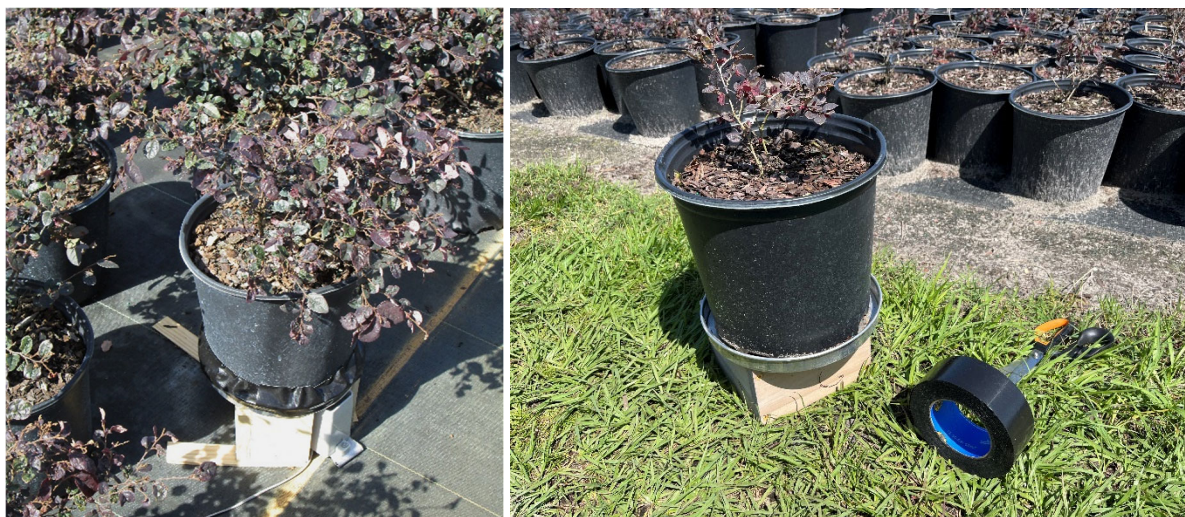
Fig. 5. For sprinkler irrigated Loropetalum at Hibernia nursery, a “skirt” taped around the pan was used to keep irrigation from directly entering the collection pan (left). A wood stand was used so the tipper could be situated inside the stand below the pan, and thus not directly intercept sprinkler irrigation water.
