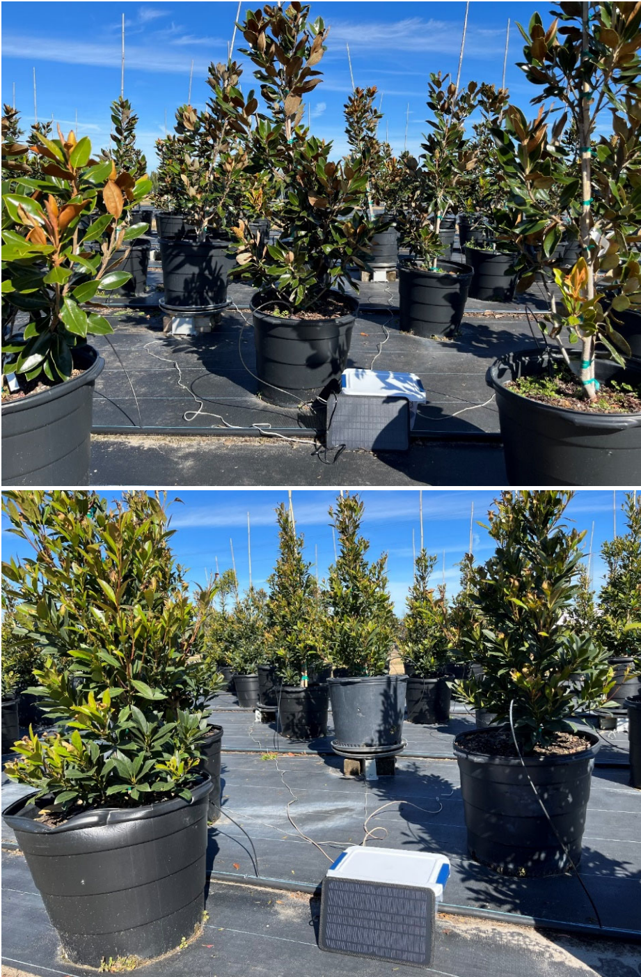
Fig. 6. Leachate from Japanese Blueberry trees (below) and Magnolia trees (above) grown in trade #15-gallon containers with spray-stake irrigation was monitored at 1-D nursery in central Florida. The Arduino housed in the plastic tote and powered with battery and solar charger was connected to four tippers to monitor container leachate using WaterTips' app. The site was initially set up in February 2022.
