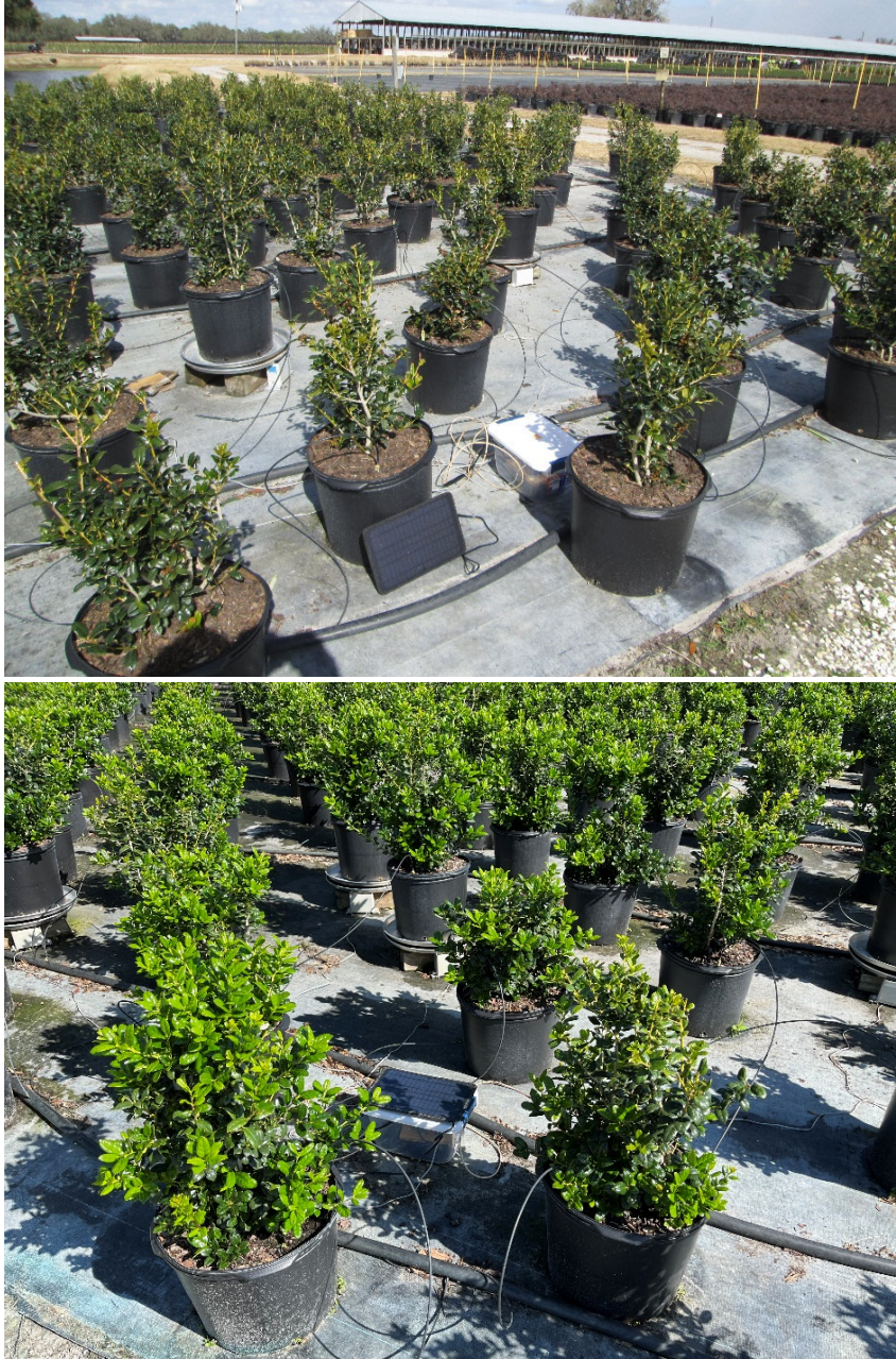
Fig. 1. Leachate from Dwarf Burford holly grown in trade #7-gallon containers with spray-stake irrigation was monitored at Hibernia nursery in central Florida. The Arduino housed in the plastic tote with white lid (lower center) was connected to four tippers to monitor container leachate using WaterTips' app. The site was initially set up in February 2022 (above) when Burford hollies were recently planted. The bottom photo was taken in May 2022 when Hibernia nursery staff recorded leachate data.
