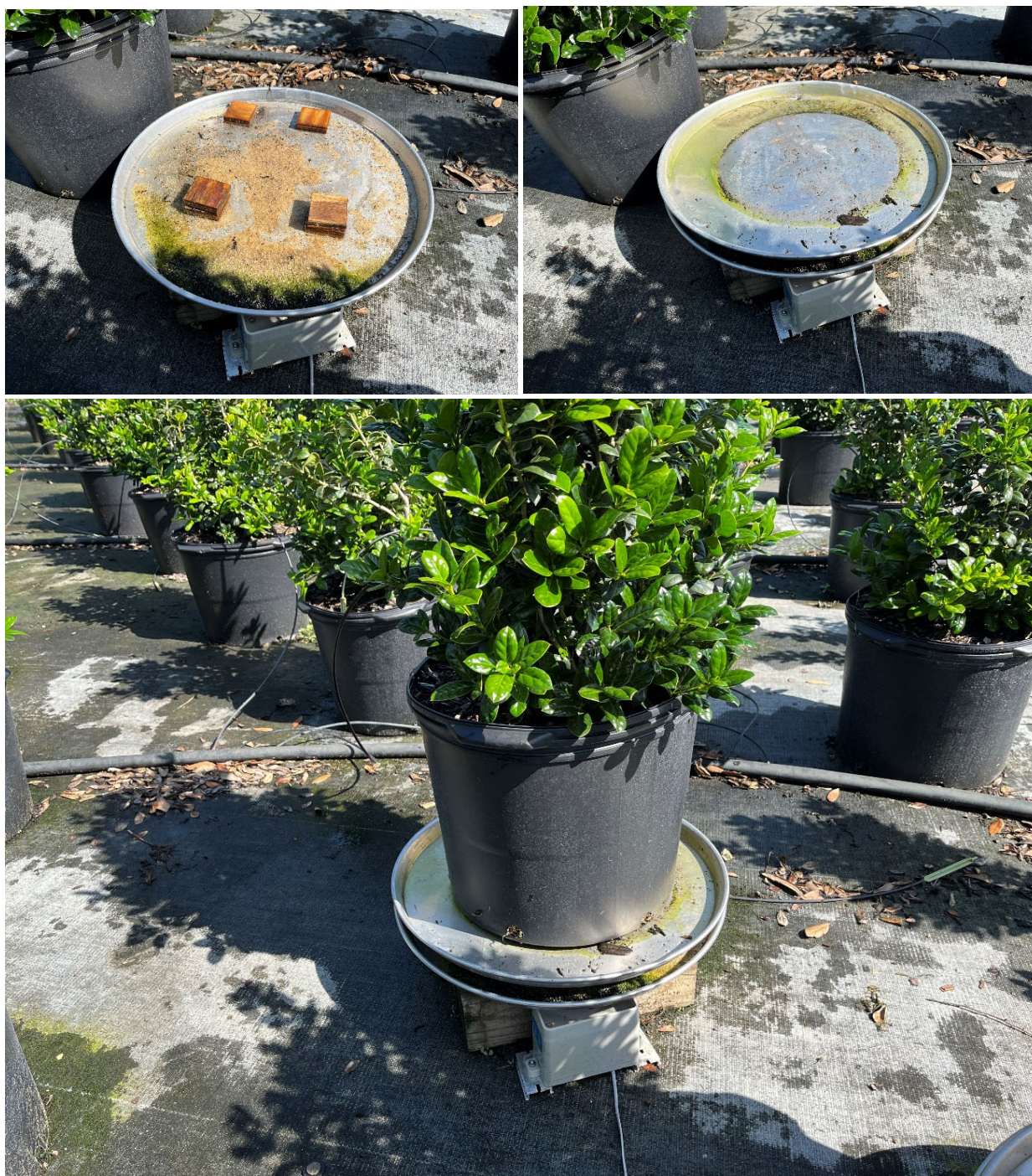
Fig. 18. Double pans were used to collect leachate and direct it to a tipping bucket rain gauge under hole in bottom pan. The bottom pan (top left) angled downward to the tipper has a handful of sand located above and around the drain hole to slow the leachate and filter out debris. The top pan (top right) is angled in the opposite direction using small wood pieces (placed on bottom pan) so that the leachate from top pan drains near the elevated edge of the bottom pan. Lower photo of Dwarf Burford holly at Hibernia nursery shows the double pans.
