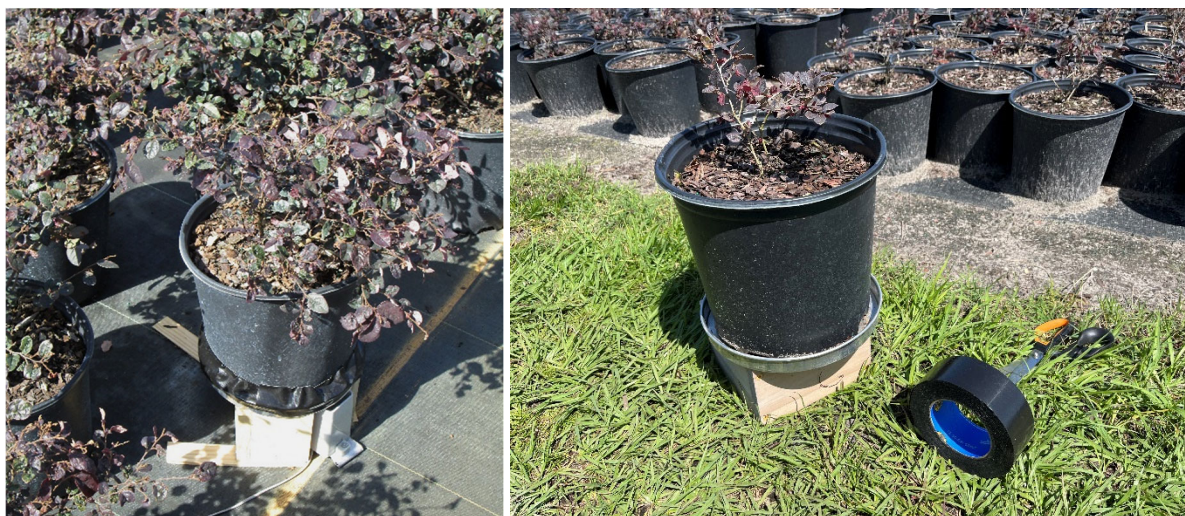
Fig. 20. For sprinkler irrigated Loropetalum at Hibernia nursery, a "skirt" taped around the pan was used to keep irrigation from directly entering the collection pan (left). A wood stand was used so the tipper could be situated inside the stand below the pan, and thus not directly intercept sprinkler irrigation water.
