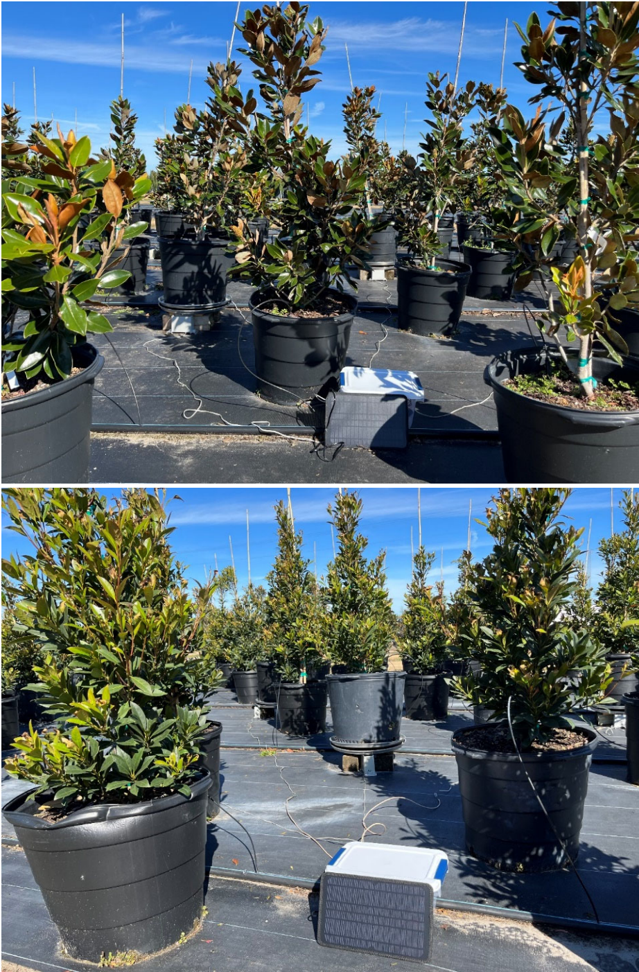
Fig. 21. Leachate from Japanese Blueberry trees (below) and Magnolia trees (above) grown in trade #15-gallon containers with spray-stake irrigation was monitored at 1-D nursery in central Florida. The Arduino housed in the plastic tote and powered with battery and solar charger was connected to four tippers to monitor container leachate using WaterTips' app. The site was initially set up in February 2022.
