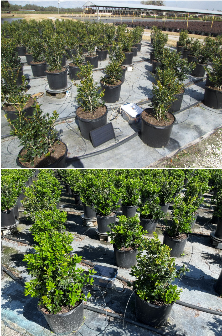
Fig. 16. Leachate from Dwarf Burford holly grown in trade #7-gallon containers with spray-stake irrigation was monitored at Hibernia nursery in central Florida. The Arduino housed in the plastic tote with white lid (lower center) was connected to four tippers to monitor container leachate using WaterTips' app. The site was initially set up in February 2022 (above) when Burford hollies were recently planted. The bottom photo was taken in May 2022 when Hibernia nursery staff recorded leachate data.
