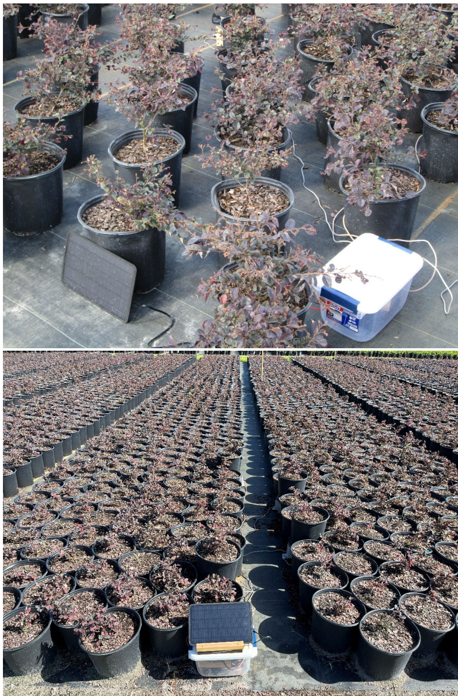
Fig. 17. Loropetalum grown in trade #3-gallon containers with sprinkler irrigation at Hibernia nursery in central Florida. The Arduino housed in the plastic tote was connected to four tippers to monitor container leachate. The above photo was taken in February 2022 when tippers were initially set up. These spaced plants were sold in March and replaced with a new Loropetalum planting that was pot-to-pot (bottom photo).
