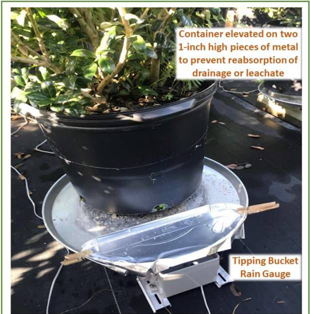
Figure 2. Seven-gallon container was placed on 17-inch pizza pan elevated 5 inches on wooden platform to direct drainage into tipping bucket rain gauge to measure leachate volume. The aluminum foil covers a layer of sand that filters out debris and slows the flow of leachate into the tipping bucket.
