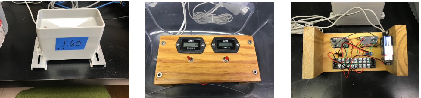
Figure 1. Tipping bucket rain gauges (left) were used to measure leachate and irrigation volume. When wired with a pulse counter (middle and right), the number of tips can be counted and converted to volume knowing the tipping bucket volume per tip (e.g. 1.5 cm 3 /tip).
